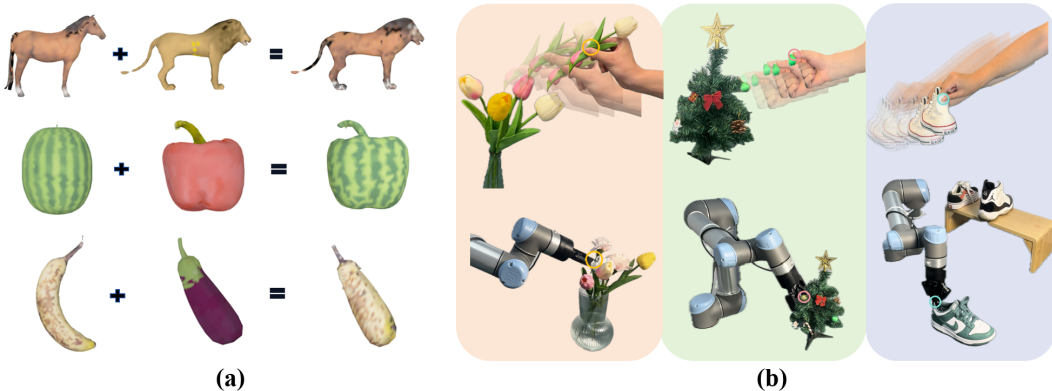
Figure 1: (a) Zero-shot color transfer between 3D assets. (b) In real-world robotic experiments, we use DenseMatcher to transfer a manipulation sequence to the robot from a single human demonstration. Circles represent the contact points in the human demo / grasping points for robot manipulation.
