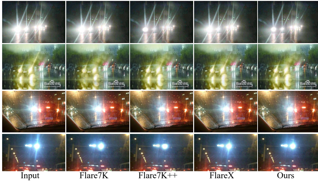
Figure 5: Visual comparison of flare removal on the test set collected from Google Image Search. The name of each column represents the dataset that is used to train Uformer.
