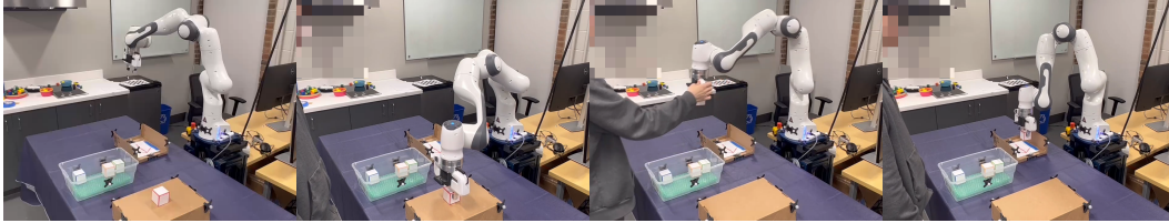
Figure 22: We shift the cube starting platform, the tunnel, and the bin. By reusing and composing the previously learned DS with task transfer, the robot is able to finish the tasks of picking, scanning, and placing without new demonstration in this new environment configuration. Also, there is human disturbance involved during the task execution.
