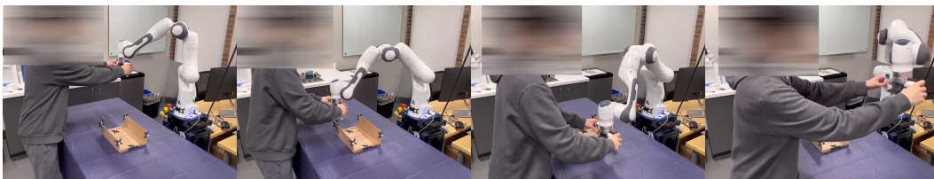
Figure 16: The human guides the end-effector for an inspection task, starting from the left side, passing through a tunnel, and stopping on the right side
