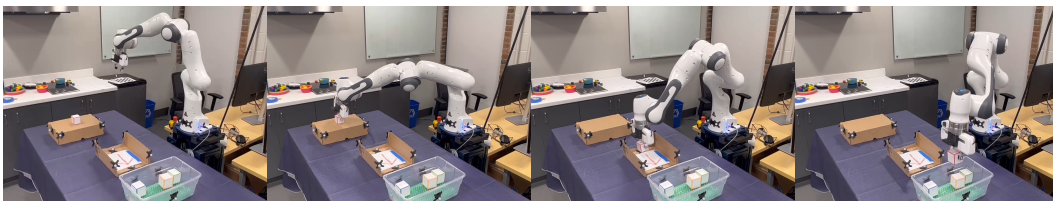
Figure 21: Composing the learned DSs with task transfer parameters from the "pick and place" and "tunnel" tasks. The robot is able to pick up a block, pass through the tunnel for scanning, and place the block in the bin. The entire motion does not require extra demonstration. Note the positions of the objects are not the same as in the original demonstrations.
