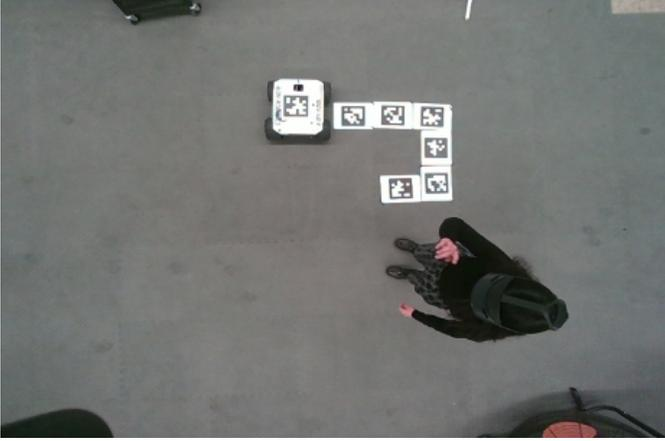
Fig. 1: System picture in which a ground rover, Microsoft HoloLens 2, and Apriltags for camera calibration is captured by an overhead camera
