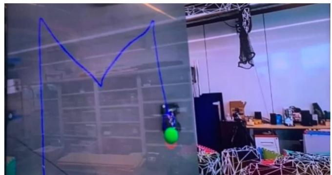
Fig. 6: This picture displays a successful execution of a system demo in which the final waypoint has just been reached. As shown in the picture, the interface allows the user to visualize the holographic interface and the physical surroundings.
