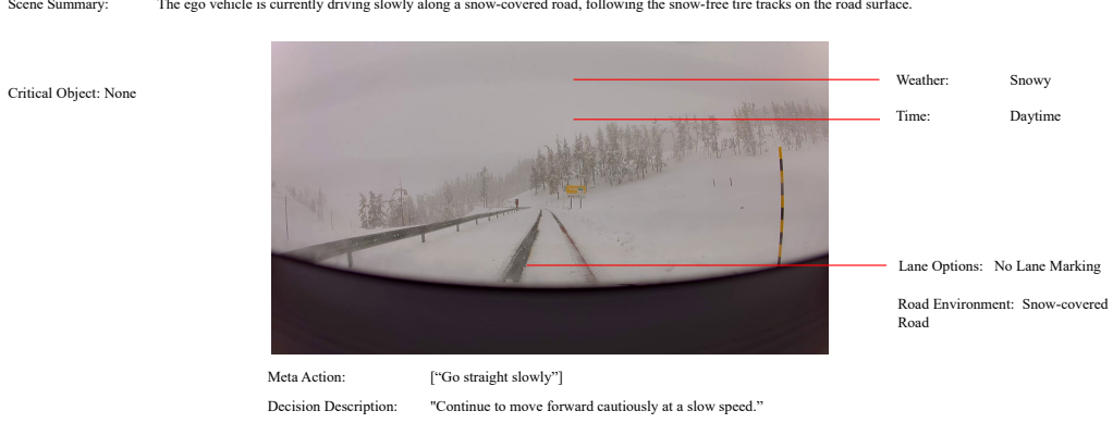
Figure 9: An example of snowfall in the SUP-AD dataset. Most of the road is covered by snow, requiring the ego vehicle to move forward cautiously by following the snow-free tire tracks.
