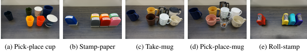
Figure 5: Overview of objects used in real-robot experiments. In each image, the single object on the left side is used during data collection, and all the objects on the right side are not seen during training. They are used for the evaluation of new object generalization in each task.
