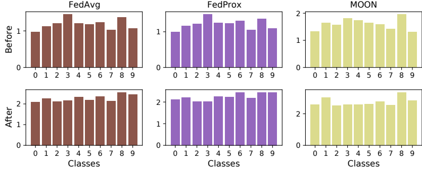
Figure 10: The classifier weight L2-norm of FedAvg, FedProx and MOON before and after applying CCVR on CIFAR-10.
