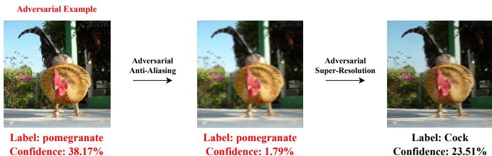
066 067 068 069 070 Figure 1: The proposed adversarial defense pipeline. We give an adversarial example of “cock” class with AutoAttack \ell_{\text{inf}} = 8/255 on ImageNet dataset. Adversarial anti-aliasing aims to eliminate adversarial perturbations, while adversarial super-resolution seeks to restore benign images from blurred adversarial examples using prior knowledge from the clean dataset.
