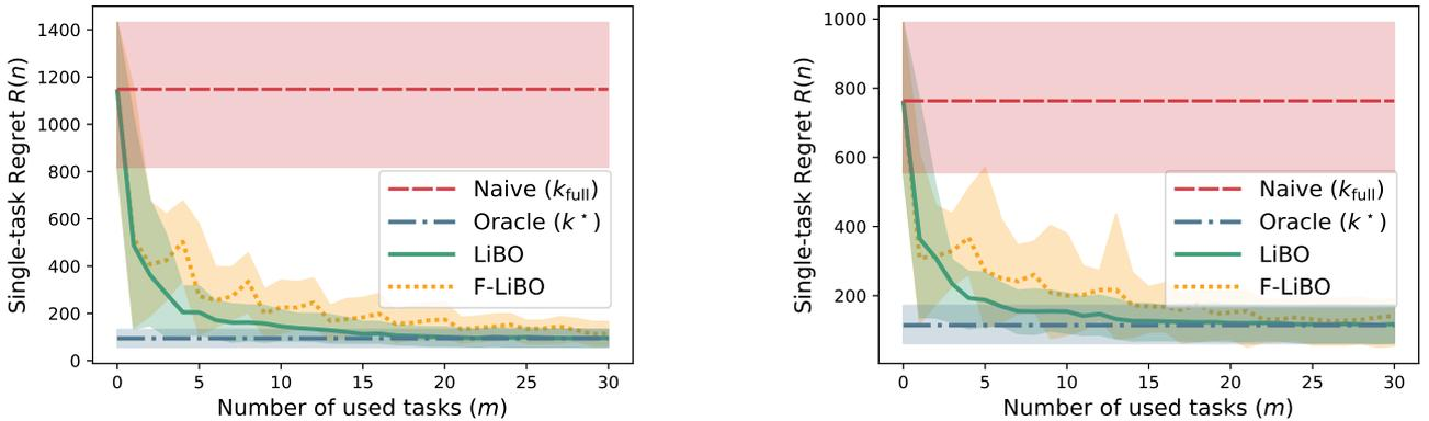
Figure 2: Single task cumulative regret of GP-UCB with meta-learned kernel  $\hat{k}$  on an increasing number of meta-training tasks. Left: base kernels constructed with 2-dimensional cosine basis. Right: base kernels constructed with 1-dimensional Legendre polynomials. The BO performance with meta-learned kernels quickly approaches oracle performance as the number of meta-training task increases.
