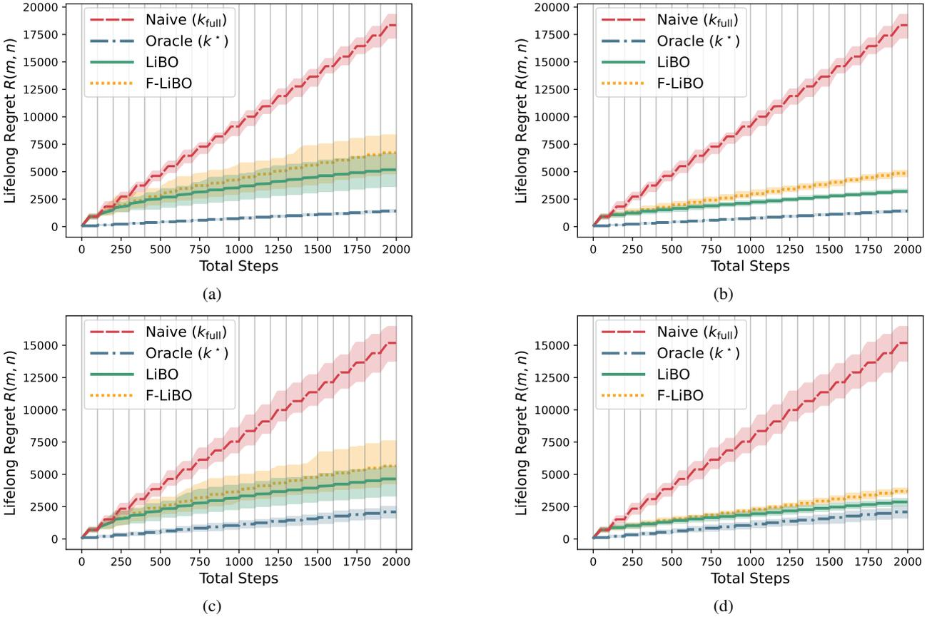
Figure 3: Lifelong regret with cosine basis (a & b) and Legendre polynomials as feature maps (c & d). In the plots (a & c) on the left, we use only the forced exploration data  $D_{1:s}^{\text{exp}}$  for meta-learning the kernel. For the plots (b & d) on the right,  $D_{1:s}$ , the data from all previous bandit interactions, is used. We observe that convergence is much faster when all interaction data is used in LiBO and F-LiBO.
