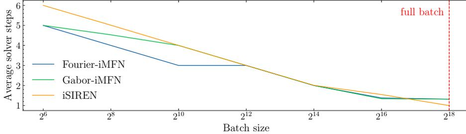
Figure 1: Average fixed-point solver steps *versus* mini-batch sizes. The average steps are taken over the last 1,000 training iterations of each model. From the figure, it can be seen that the required solver steps is inversely related to the batch size. However, only when the batch size is sufficiently large ( $> 2^{16}$ ) can the majority of the fixed-points converge in 1 step (average solver steps  $< 1.5$ )
