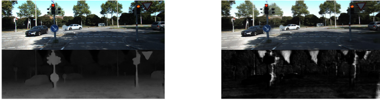
(a) Input center image and disparity map (b) Output panned image and occlusion map
