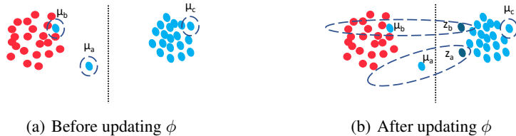
Figure 3: The Gaussian distribution within one standard deviation \sigma away from mean, shown before and after updating \phi . The dotted circles represent the \sigma of the sample inside it. Red and blue dots represent training samples belonging to two different classes in the representation space. The dotted line is the decision boundary in the space. Let’s take the two mis-classified training samples \mu_a , \mu_b and the correctly classified \mu_c as examples. (a), before updating \phi , the \sigma s of both correctly and wrongly located samples are initialized with a small value. (b), after updating \phi , \sigma of mis-classified samples are much larger. Because the proto-loss for calibration will move z , sampled from \mathcal{N}(\mu, \text{diag}(\sigma \odot \sigma)) , to be as close to the correct class center as possible.
