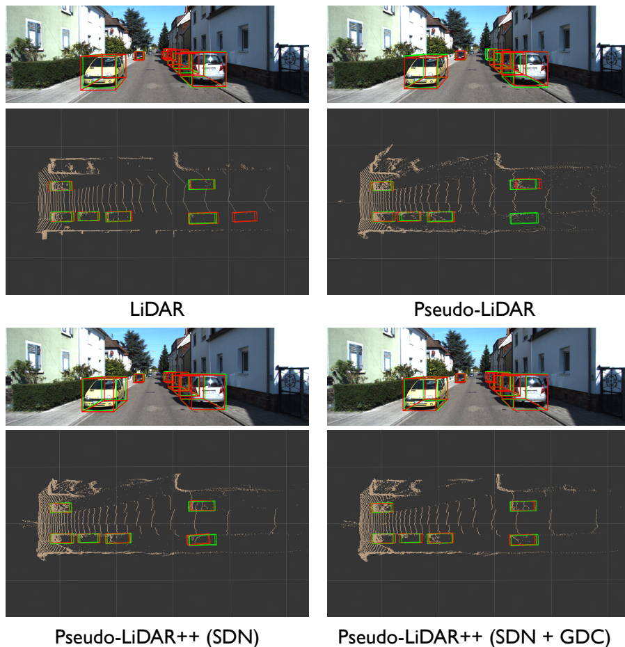
Figure 9: Qualitative Comparison. We show the detection results on a KITTI validation scene by P-RCNN with different input point clouds. We visualize them from both frontal-view images and bird’s-eye view (BEV) point maps. Ground-truth boxes are in green and predicted bounding boxes are in red. The observer is at the left-hand side of the BEV map looking to the right. In other words, ground truth boxes on the right are more faraway (i.e. deeper) from the observer, and hence hard to localize. Best viewed in color.
