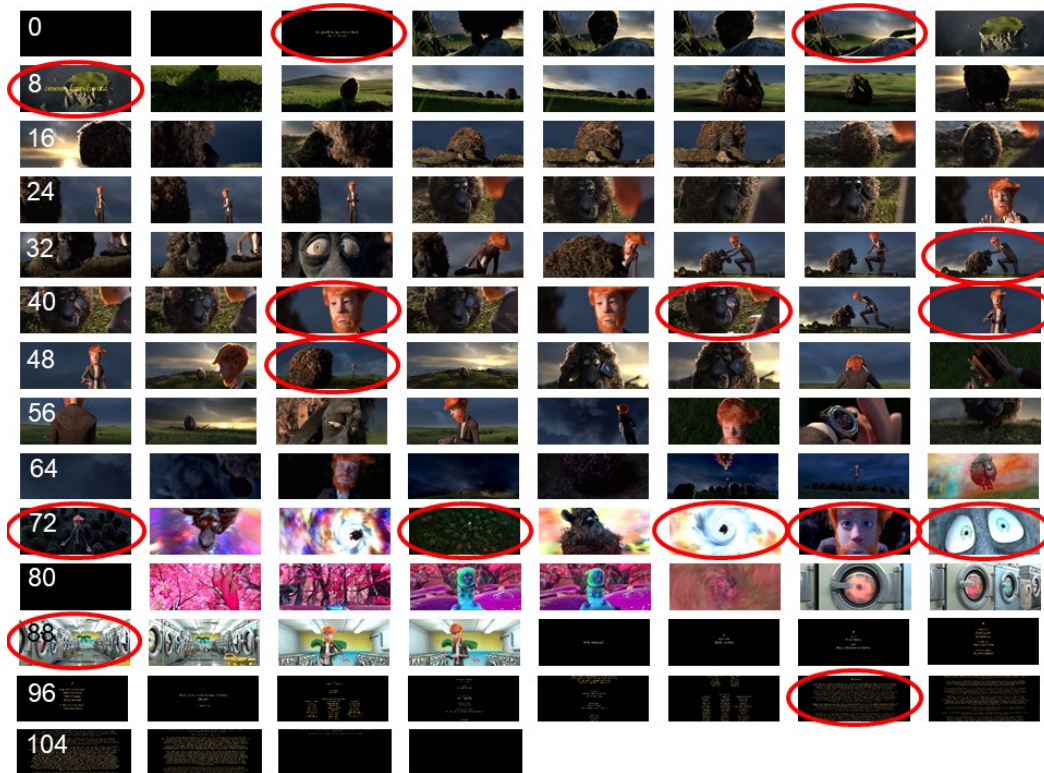
Figure 2: ILS-SUMM selection in Cosmos Laundromat movie from OSTD data set. The middle frame of shot is presented. A red circle denotes the shots that were chosen by ILS-SUMM algorithm.
