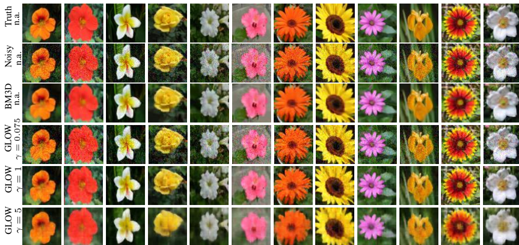
Figure 14: Image Denoising — Visual comparisons under the Glow prior, and BM3D at noise level \sigma = 0.1 on (within-distribution) test set Flowers images. Under Glow prior, the best performance is obtained with \gamma = 1 . Note that the Glow prior with \gamma = 1 also gives a sharper image than BM3D.
