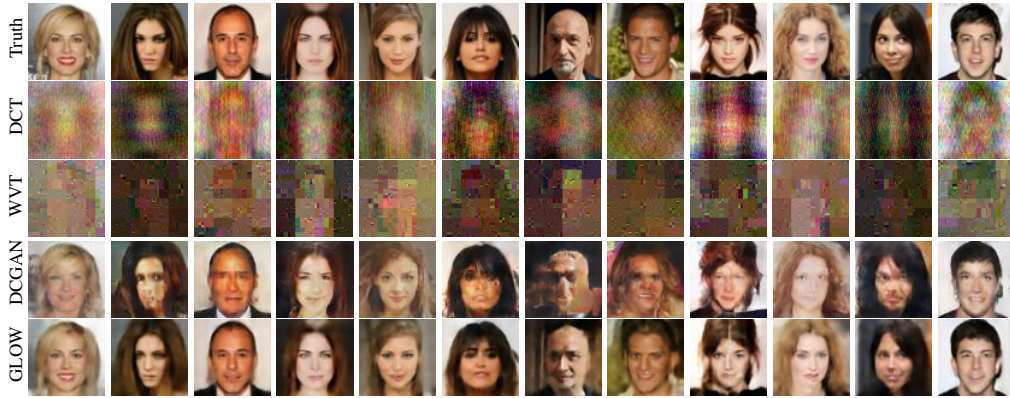
Figure 23: Compressed sensing visual comparisons — Recoveries on (within-distribution) test set images with a number m = 400 ( \approx 3\% ) of measurements under the Glow prior, the DCGAN prior, LASSO-WVT, and LASSO-DCT at a noise level \sqrt{\mathbb{E}\|\eta\|^2} = 0.1 . In each case, we choose values of the penalization parameter \gamma to yield the best performance among the tested values. We use \gamma = 0 for both DCGAN, and Glow prior and \gamma = 0.01 for LASSO-WVT, and LASSO-DCT, respectively.
