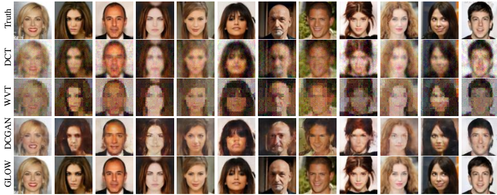
Figure 27: Compressed sensing visual comparisons — Recoveries on (within-distribution) test set images with a number m = 2500 ( \approx 20\% ) of measurements under the Glow prior, the DCGAN prior, LASSO-WVT, and LASSO-DCT at a noise level \sqrt{\mathbb{E}\|\eta\|^2} = 0.1 . In each case, we choose values of the penalization parameter \gamma to yield the best performance among the tested values. We use \gamma = 0 for both DCGAN, and Glow prior and \gamma = 0.01 for LASSO-WVT, and LASSO-DCT, respectively.
