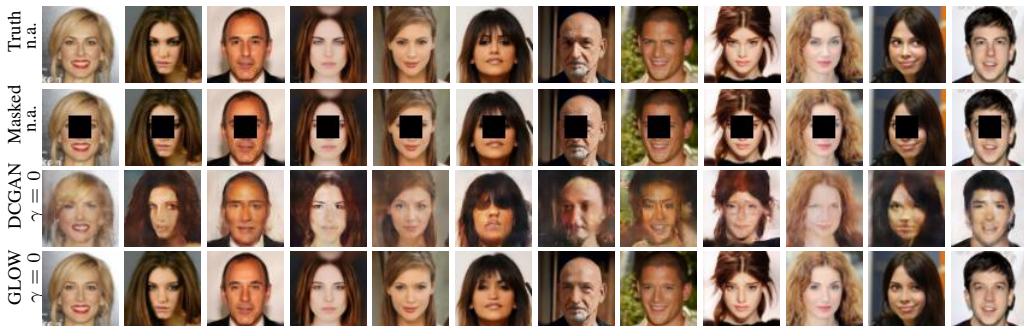
Figure 48: Image inpainting results on CelebA test set. Masked images are recovered under DCGAN prior and Glow prior. Recoveries under DCGAN prior are skewed and blurred whereas Glow prior leads to sharper and coherent inpainted images. For both Glow and DCGAN, we set \gamma = 0 .
