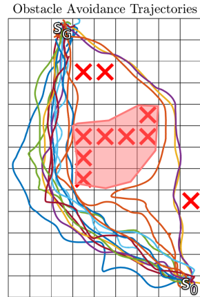
Figure 1: Human trajectories overlaid on a grid world MDP. The shaded region represents an obstacle in the human’s environment, and the red “X”s represent learned constraints.
