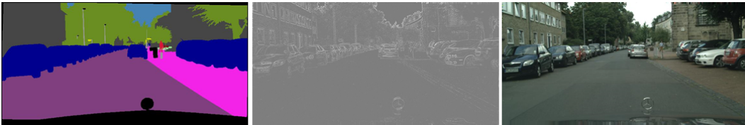
Figure 2: example of the images for training the model. Left is the semantic map. Middle is the edge map extracted from the real image. Right is the real image being used by the discriminator for adversarial training. Please note that the real image is not used by the generator neither at training nor at test time, but only its edge map. The main issue in the CG2real model compared to the image to image models is that the simulator's image is available to the generator at test time. We thus use the simulator's image to extract the edge map allowing the generator to generate the necessary fine details in the output image.
