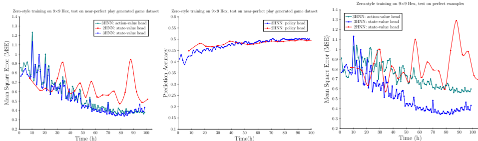
Figure 2: AlphaZero-2HNN versus AlphaZero-3HNN learning progresses measured in training time. MCTS-3HNN performs 800 iteration MCTS faster than MCTS-2HNN because it uses an expand threshold 10, while MCTS-2HNN uses threshold 0. Consequently, 3HNN leads to faster AlphaZero learning than that of 2HNN. Note that for the random play examples, because final move is random, we only test the value error on these examples (rightmost).
