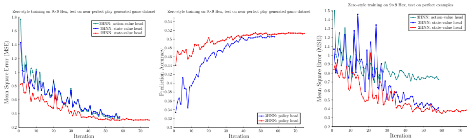
Figure 4: AlphaZero-2HNN versus AlphaZero-3HNN. AlphaZero-3HNN used a MCTS with expand threshold 1. Upon writing, only 60 iterations are finished for AlphaZero-3HNN.
