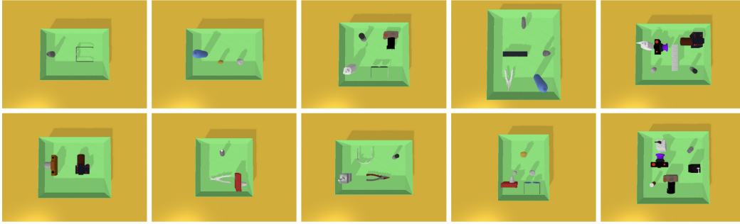
Figure 11: Example configuration of 3D shapes that enables the robot place each object in a given sequence without colliding into other objects already placed. All the bottles, dispensers, and bowls affords only side grasps.
