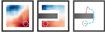
Figure 5: (left and middle) Difference in learned global metric on Open Room and C-Maze. The goal used to query the value map is indicated by the dashed circle. (right) shows the agent getting around the wall with the learned embedding (blue), whereas an Euclidean planner gets stuck.
