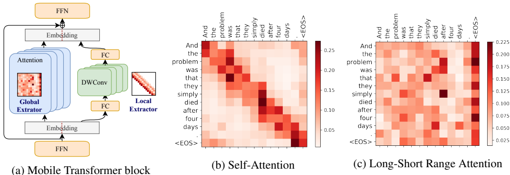
Figure 3: Model architecture (a) and the visualization of attention weights. Conventional attention (b) put too much emphasizes on short-range relationship modeling (diagonal structure). We filtered the short-range relationship modeling by a convolutional branch which efficiently models locality, so that the attention branch can evenly focus on short-range and long-range modeling (c).
