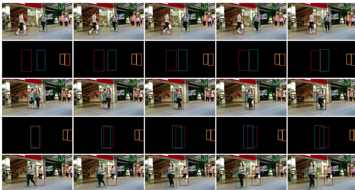
FIGURE 9: Camera blackout experiment on a pedestrian street scene from the MOTChallenge dataset without ego-motion. Subsequent frames are displayed going from top left to bottom right. Shown are the inputs to the model (some of them being black frames, i.e. arrays of zeroes) and bounding boxes predicted by MOHART (coloured boxes). This scene is particularly challenging as occlusion and missing sensor input coincide (fourth row).
