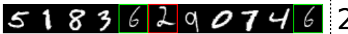
Figure 5: MNIST recall & classification. Given a random sequence of images followed by a repeat (green), output the class of the next image (red).
