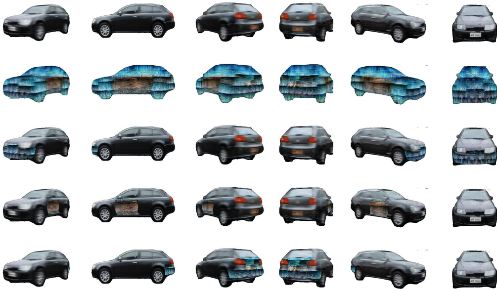
Figure 3: First row: the initial SUV-type vehicle. Second row: the trained full-part adversarial example using the SUV-type vehicle. Third row to the fifth row: The results of full part adversarial texture transfer to the front part, side part, and rear part.
