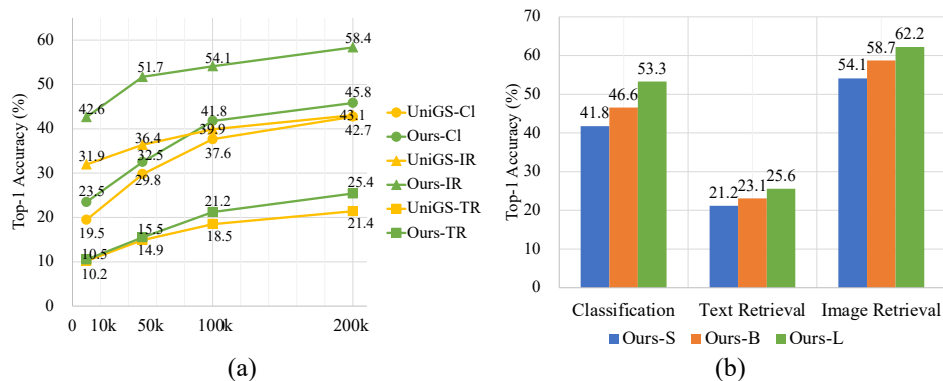
Figure 3: Analysis on scaling up the model. (a) Top-1 accuracy on Objaverse dataset with different scales of training data. We abbreviate classification as CI , image retrieval as IR and text retrieval as TR . (b) Top-1 accuracy on Objaverse dataset with different backbone setups.
