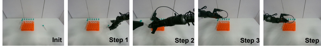
TubeRack : “Insert the tube on the table surface into an empty slot of the rack.” (Step1) Pick up the tube. (Step2) Reorient the tube and pass it to the other gripper. (Step3) Insert the tube into the rack. (Step4) Release the tube.
