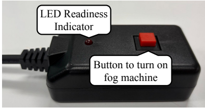
Figure 3. The handheld fog machine controller has an LED to indicate the machine’s readiness for producing fog and a red button to operate the fog machine, preventing autonomous fog production.
