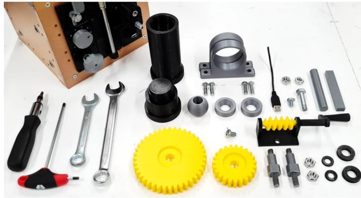
Figure 2: The Generic Assembly Box consists of 11 standard parts and 25 non-standard parts and requires 4 different standard tools during assembly.
