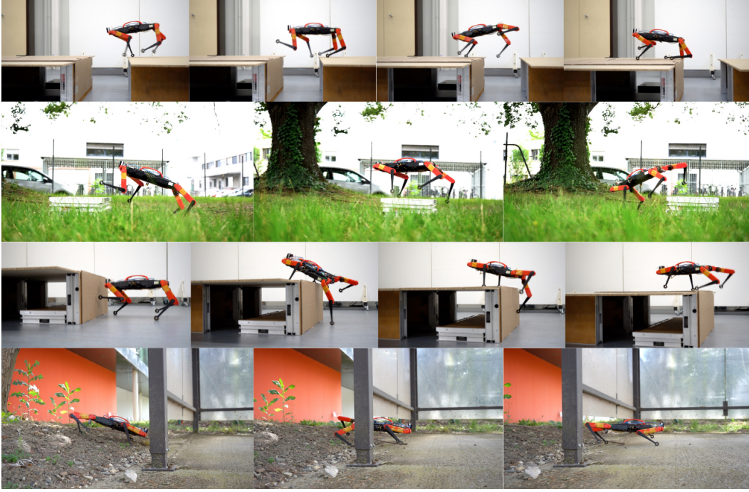
Figure 6: Solo-12 performing agile locomotion skills in diverse indoor and outdoor environments such as climbing high steps, leaping over gaps, and crawling under obstacles.
