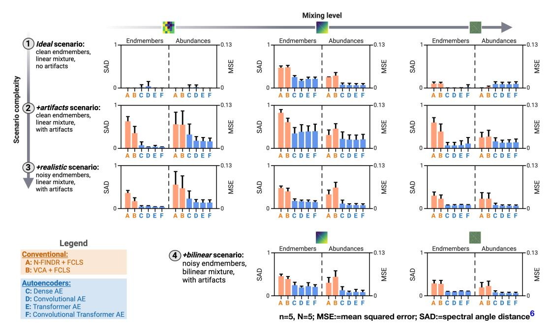
**Hyperspectral unmixing** aims to resolve mixed signals by identifying the individual components present (*endmembers*) and quantifying their proportions (*fractional abundances*).
