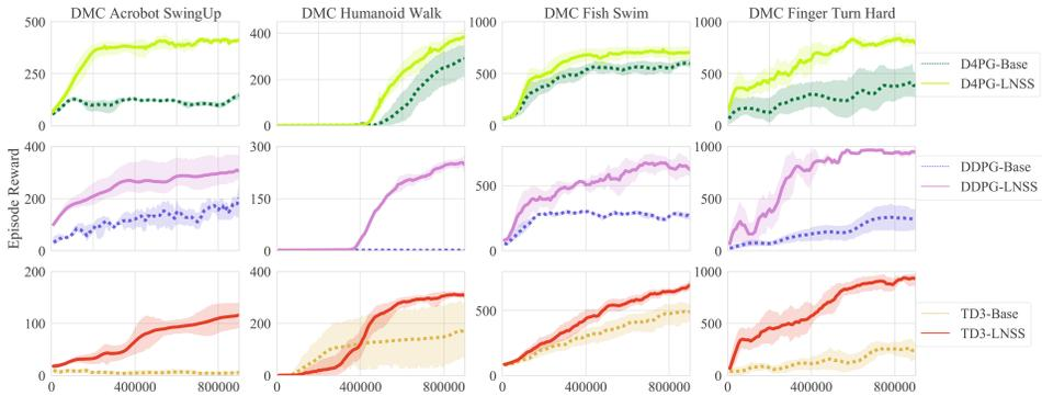
Figure 7: Systematic evaluation of LNSS piggybacked on three DRL algorithms (DDPG, D4PG, TD3) in DMC environments without reward noise. The shaded regions represent the 95 % confidence range of the evaluations over 10 seeds. The x-axis is the number of steps.
