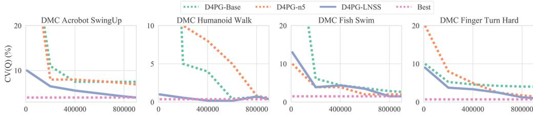
Figure 12:  $cv(Q)$  (coefficient of variation of  $Q$  value, the lower the better) of D4PG in DMC environments. Results are averaged over 10 seeds. The x-axis is the number of steps.
