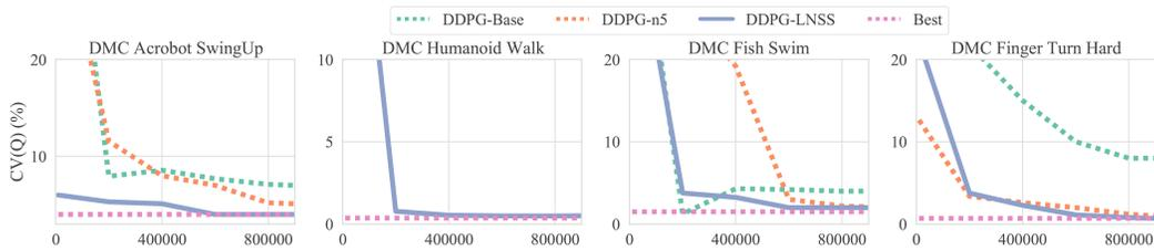
Figure 13:  $cv(Q)$  (coefficient of variation of  $Q$  value, the lower the better) of DDPG in DMC environments. Results are averaged over 10 seeds. The x-axis is the number of steps.
