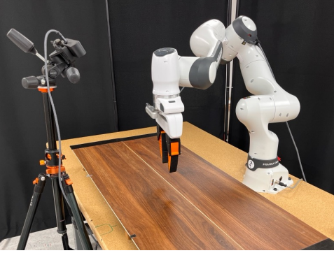
Fig. 1: Our hardware experiment setup, we use a Franka Research 3 robot, with a UMI gripper. The RealSense D435 wrist camera, and Zed mini 2i third person camera are placed as shown.
