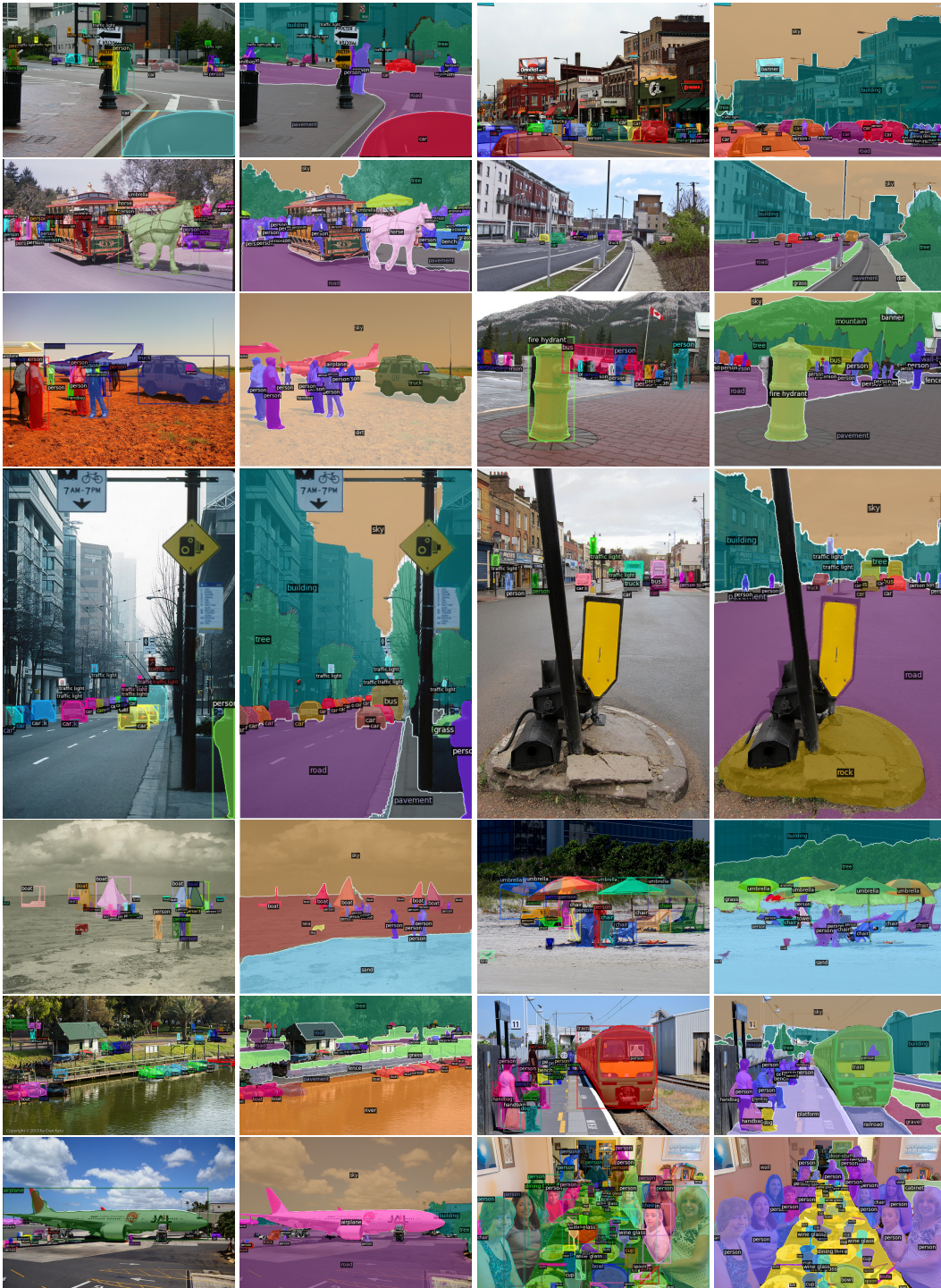
Figure C: Qualitative results for object detection, instance segmentation, and panoptic segmentation generated by SimPLR using ViT-B as backbone on the COCO val set. In each pair, the left image shows the visualization of object detection and instance segmentation, while the right one indicates the panoptic segmentation prediction.
