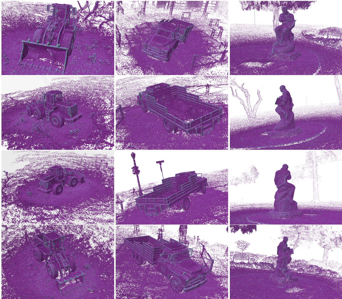
Figure A.4. Curvature computed by ours (M+N) on the Tanks and Temples dataset. The result is visualized in different views. Our method can well estimate the curvature for both the high curvature points lying on the edges and low curvature points lying on the smooth surface. The figure is visualized using the viridis colormap.
