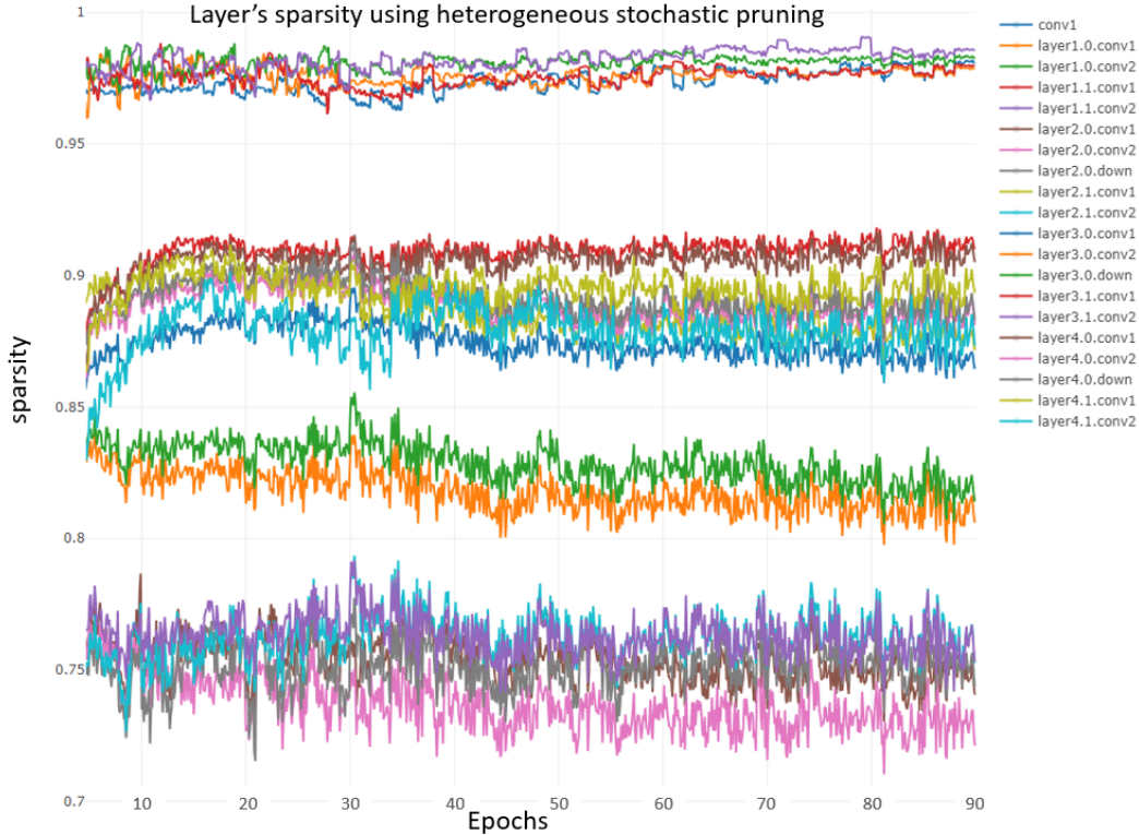
Figure A.19: Actual sparsity of the different layers of ResNet18 trained on ImageNet using heterogeneous stochastic pruning. The desired sparsity was 92% and the overall achieved one is 91.5%, the minimum cosine similarity for blocks 3 & 4 was 0.98 and for block 2 was 0.95, and the maximum allowed sparsity for the rest of the layers (block 1 and "conv1" before the first block) was 0.98. Notice that the high sparsity levels were induced on the first block and "conv1", and that some of the layers, especially from block 2, had much lower sparsity levels in order to preserve its cosine similarity. For this experiment the validation accuracy was less than 1% degradation from baseline, compared to over 3% degradation for the homogeneous algorithm at similar sparsity level.
