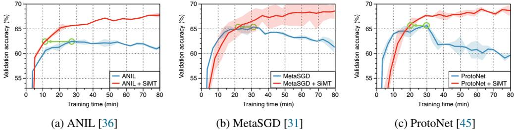
Figure 5: Comparison of the computational efficiency between the base adaptation subroutine algorithm and SiMT: we compare the accuracy of mini-ImageNet 5-shot classification (on Conv4) under the same training wall-clock time. The solid line and shaded regions represent the mean and standard deviation, respectively, across three runs.
