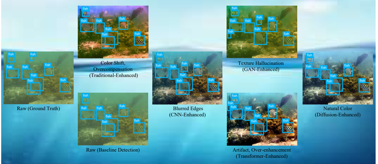
Figure 1: Qualitative comparison of UIE methods and their effects on OD. The raw image and its detection result serve as a baseline. Each enhanced version—Traditional WB (Hsu & Cheng, 2021a), CNN-based PRWNet (Huo et al., 2021), GAN-based WaterGAN (Li et al., 2017a), Transformer-based AutoEnhancer (Tang et al., 2022), and Diffusion-based UIEDP (Du et al., 2025)—introduces distinct visual changes, illustrating how UIE alters image statistics and influences detection performance.
