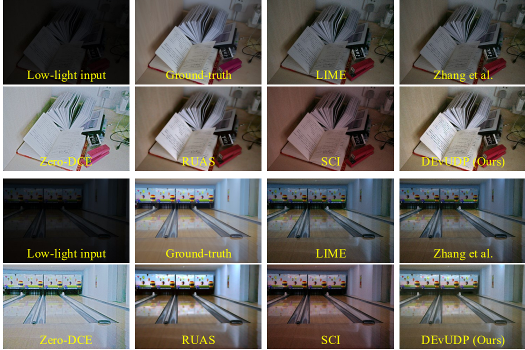
Figure 4: Visualization comparison between our method and several optimizing-based/zero-reference data-based methods. From left-top to right-bottom: low-light input, ground-truth, LIME (Guo, 2016), Zhang et al. (Zhang et al., 2019), Zero-DCE (Guo et al., 2020), RUAS (Liu et al., 2021), SCI (Ma et al., 2022) and Ours. Clearly, the enhanced results of our DEvUDP are more natural.
