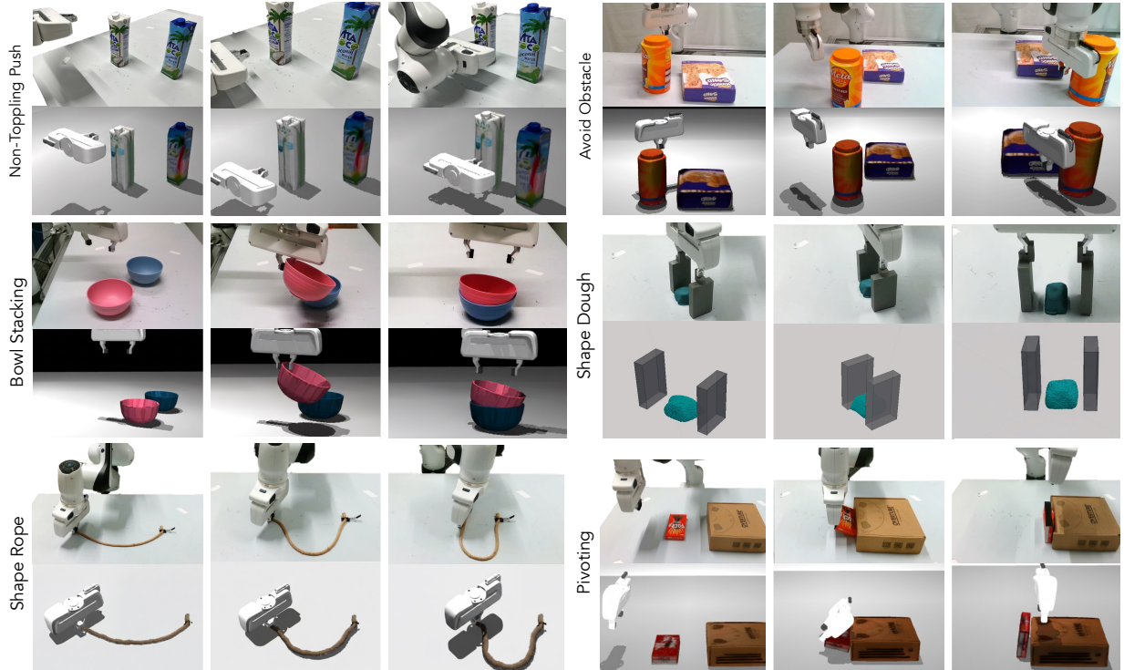
Fig. 5: Qualitative results. The figure shows the initial state, execution progress, and final state for four tasks in both the real world (top) and the simulation (bottom). By leveraging VLM’s powerful generalization, rendered simulation images can guide VLM’s test-time reasoning for action planning despite the visual sim2real gap.
