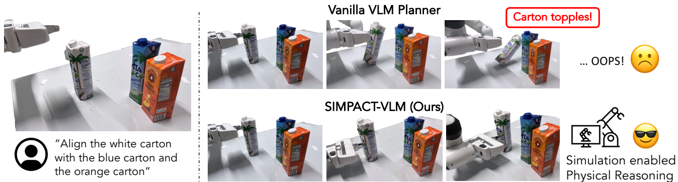
Fig. 1: Simulation-Enable VLM Action Planning. Given a single RGB-D image and a language task description ( left ), our method efficiently constructs a physics simulator that enables test-time VLM reasoning with physical grounding. This physically grounded reasoning allows the robot to succeed in fine-grained manipulation tasks ( bottom ), outperforming a vanilla VLM planner ( top ) that lacks awareness of physical dynamics.
