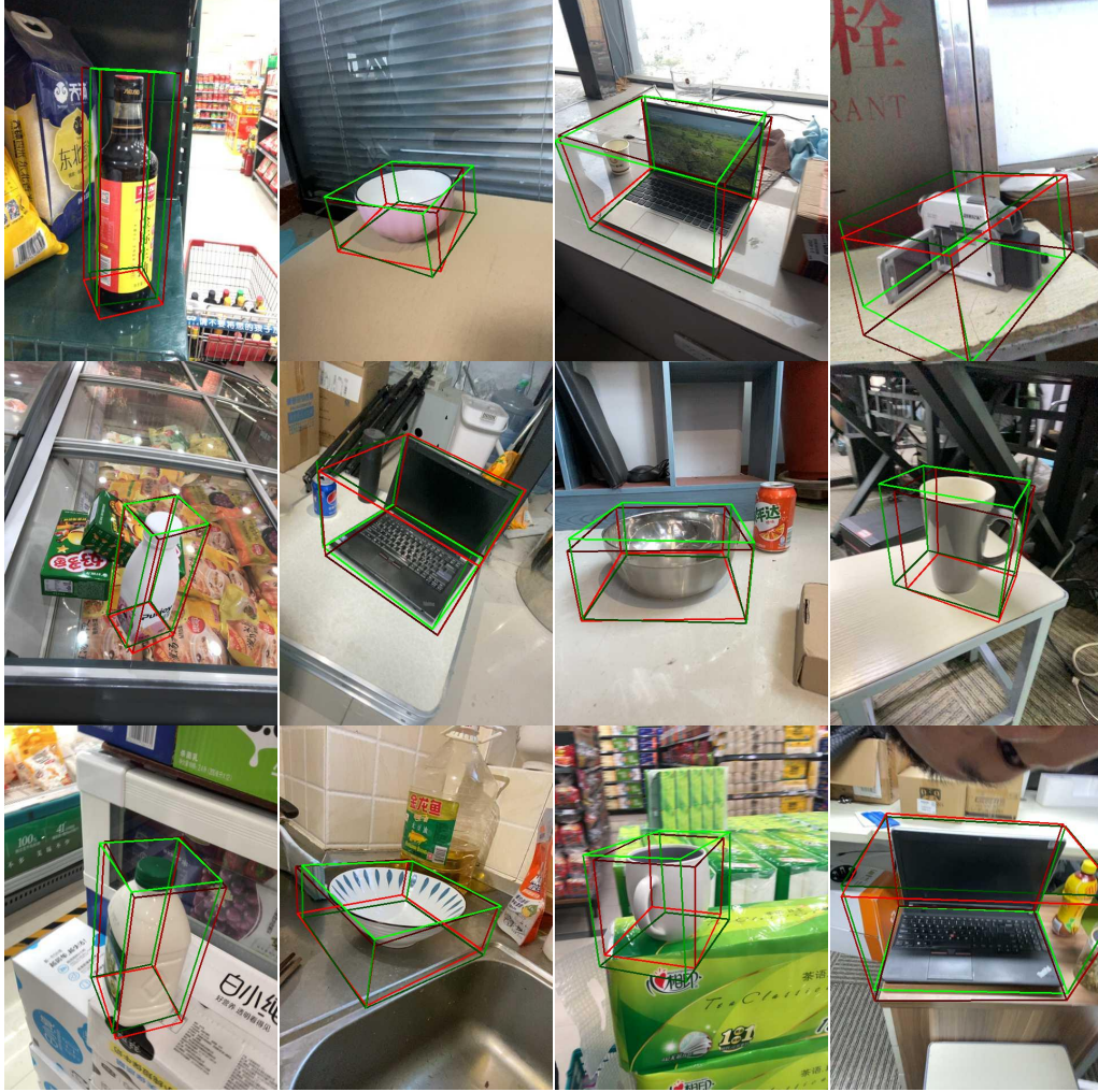
Figure 6: Visualization Results on Wild6D test set. Red 3D bounding boxes denote the ground truth, and the green boxes are estimation results via our proposed method.
