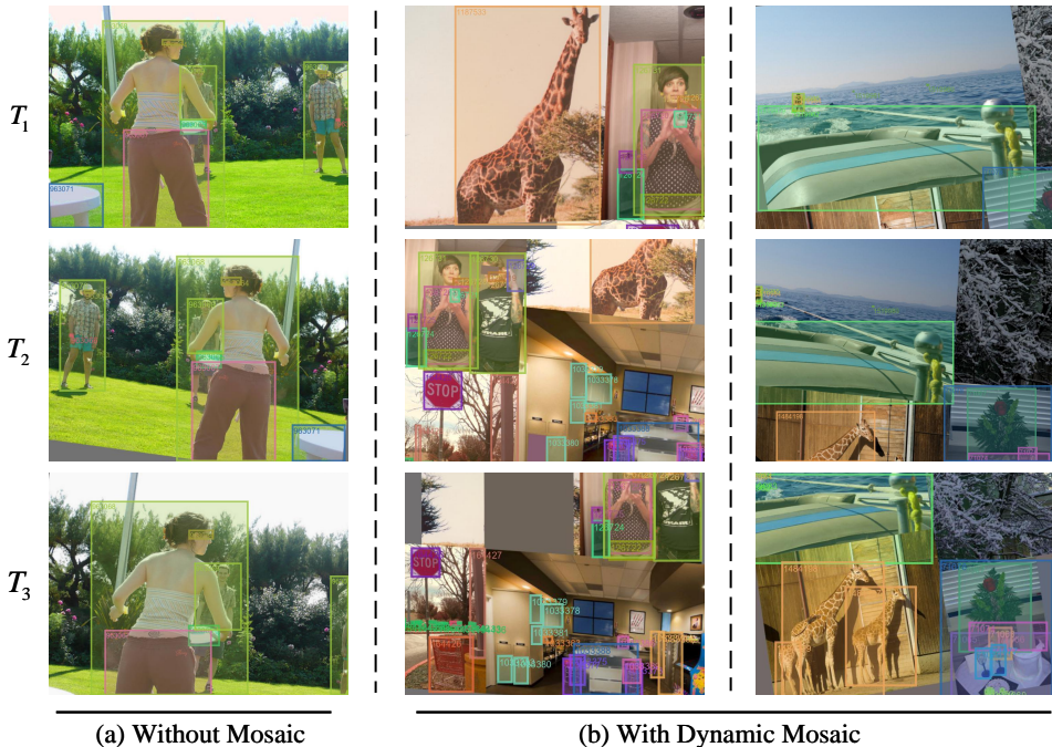
Figure 6: OVTR data augmentations visualization. From the images, it can be observed that Dynamic Mosaic augmentation introduces relative motion and relative size changes between targets, while the positional swapping of images simulates target crossing paths. Additionally, the bottom-center image illustrates a random occlusion applied to a giraffe.
