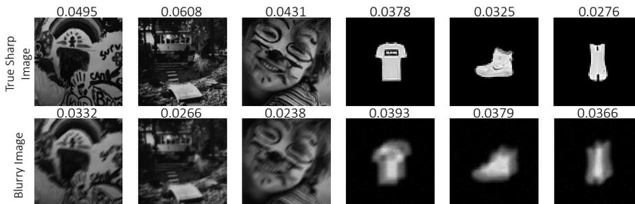
Figure 10: **Total variation (TV) values for the different true sharp images and blurry images used.** TV values for the true images (row 1) and blurry images (row 2). Note that the TV value is being used as  $-\log p(x)$ . Therefore a higher TV value indicates that an image is less likely.
