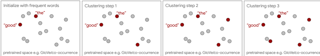
Figure 2: Initialization strategies for anchor objects combining ideas from frequency and k -means++ clustering algorithms. Clustering initialization picks anchors to span the space of all objects.
