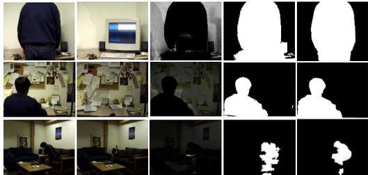
Figure 4: Wallflower dataset; first column frames of original videos; Estimated backgrounds are shown in the second column; Difference and threshold images are shown in column three and fourth respectively. Fifth column shows the enhanced images after applying morphological operations.
