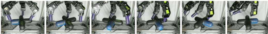
Figure 1: We present a dynamical distance learning (DDL) method that can learn a 9-DoF real-world dexterous manipulation task directly from raw image observations. DDL does not assume access to the true reward function and solves the 180 degree valve-rotation task in 8 hours by relying only on 10 human-provided preference labels.
