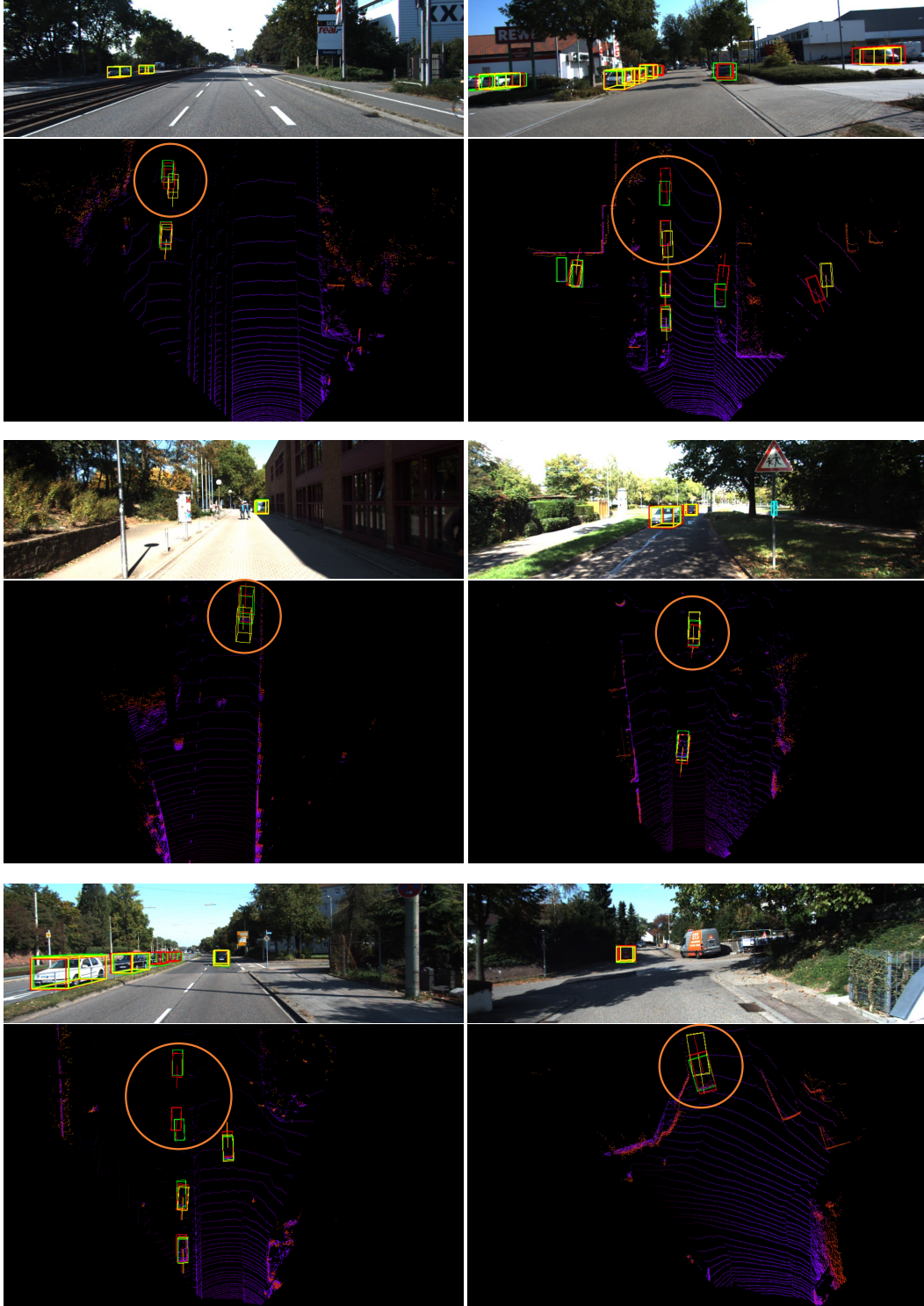
Figure 5: Comparison of our MonoHBD and MonoDTR [8] on the KITTI validation set. The green bounding boxes represent the ground truth boxes. The red , yellow boxes denote the prediction of our model and MonoDTR, respectively. Best viewed in color and zoom-in.
