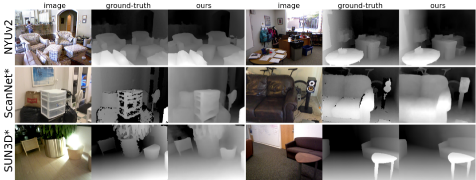
Figure 4: Visualization of predicted depth maps on NYU, ScanNet, and SUN3D. On ScanNet and SUN3D (marked with *) we show the results of the model trained only on NYU data.
