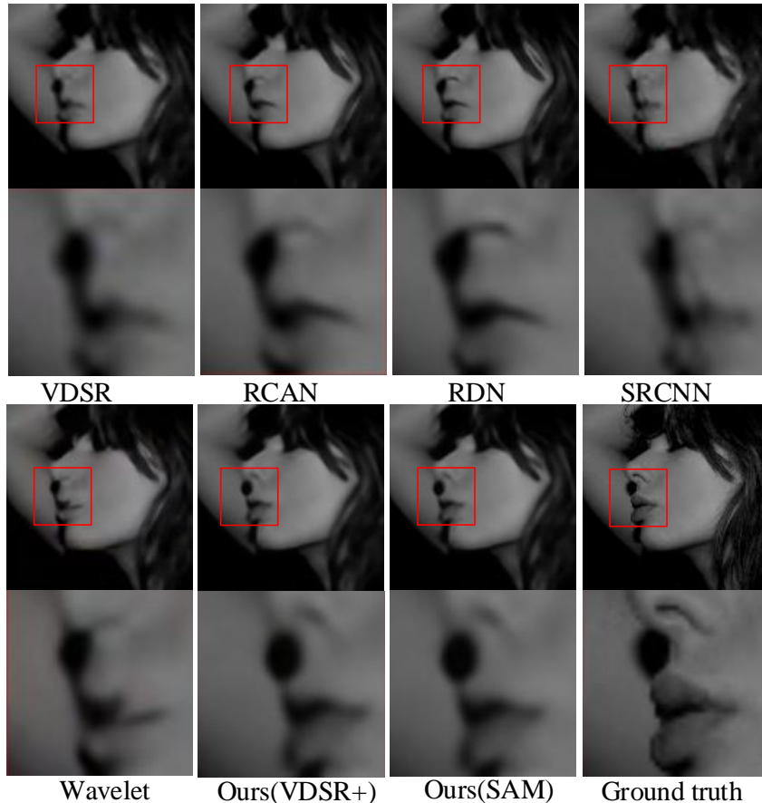
Figure 9: Comparison of state-of-the-art methods on left facial pose:magnification factor \times 4 and the input resolution 32 \times 32 .
