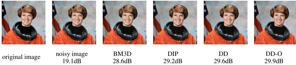
Figure 2: Denoising with BM3D and various convolutional generators. The relative ranking of algorithms is representative and maintained on a large test set of images. DIP and DD-O are over-parameterized generators and with early stopping outperform the BM3D algorithm, the next best method that does not require additional training data.
