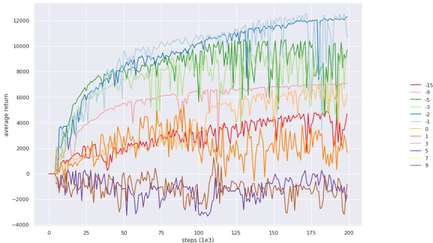
Figure 2: POUM with different subjective risk preference values on HalfCheetah-v2 environment. The moderate risk yields the best return while too much risk (either too high or too low) will harm the agent in getting good results. We use the same settings of HalfCheetah-v2 environment as presented in Appendix A.2.3 excluding risk-preference values
